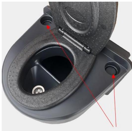
Next, you need to decide which side to run the ventilation pipe. There are ready-made places for the pipe to exit on both sides of the toilet seat. Once you've made your selection, cut a hole for the ventilation pipe on that side. A knife can be used for cutting, as the cutting seam is already thinned.
